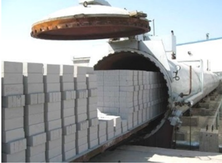
Figure 2: The 20m long steel cylinder act as an Autoclave
