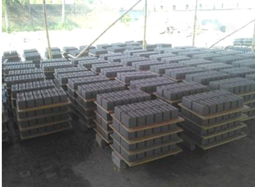
Figure 3: The stacking of Calcium Silicate Bricks
